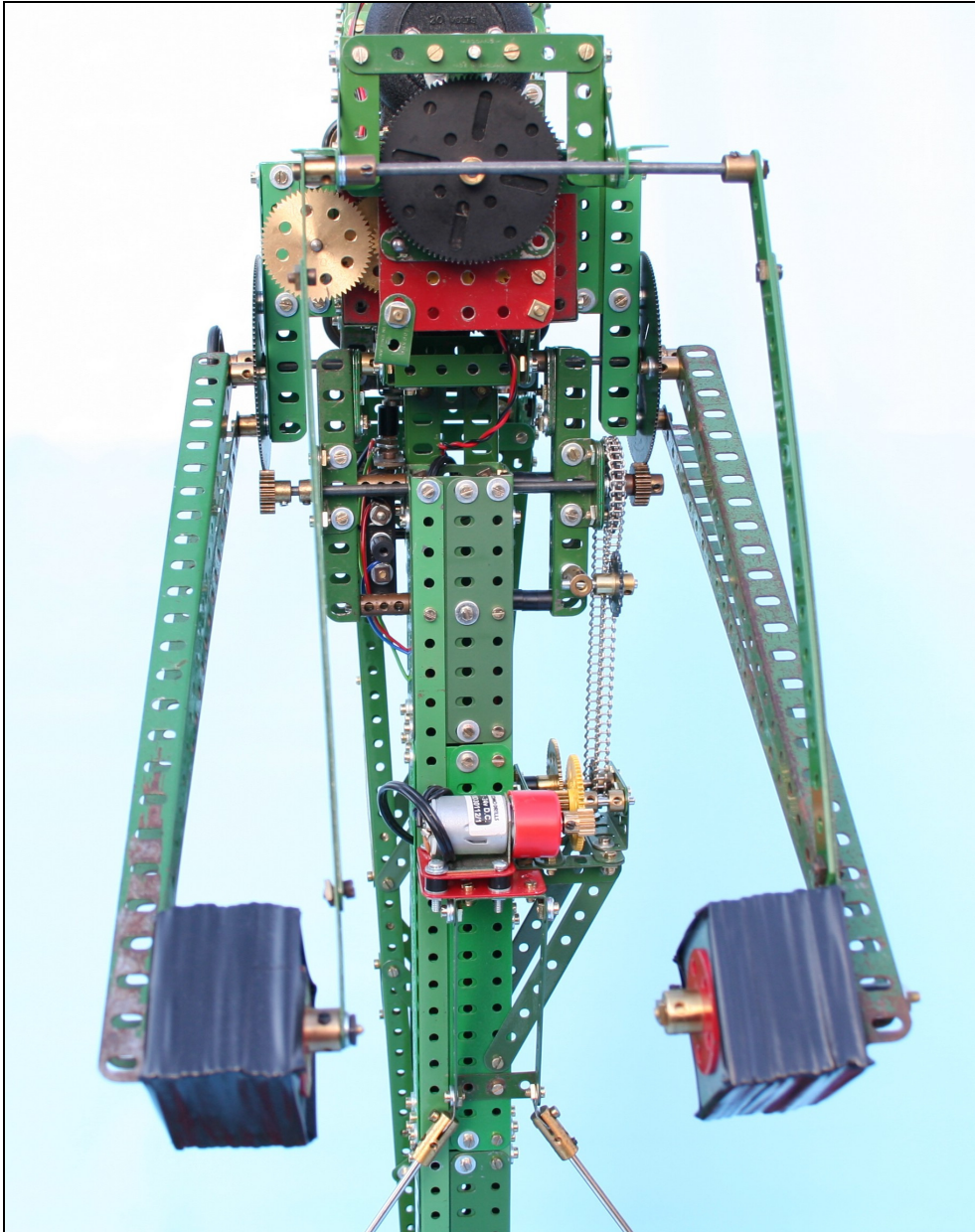
Figure 7 Rear view of revised counterweight arrangement
